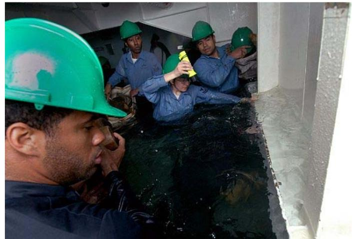
**NORFOLK, Va.** - Sailors place plugs in the hull of the USS Buttercup during a training exercise. Norfolk area Sailors and Coast Guardsmen test their damage control skills aboard the USS Buttercup during general shipboard damage control training at the Naval Station Norfolk. Once a month, Mid-Atlantic Region Sailors and Coast Guardsmen test their damage control skills aboard Buttercup, a training simulator that recreates a sinking ship. **11**
